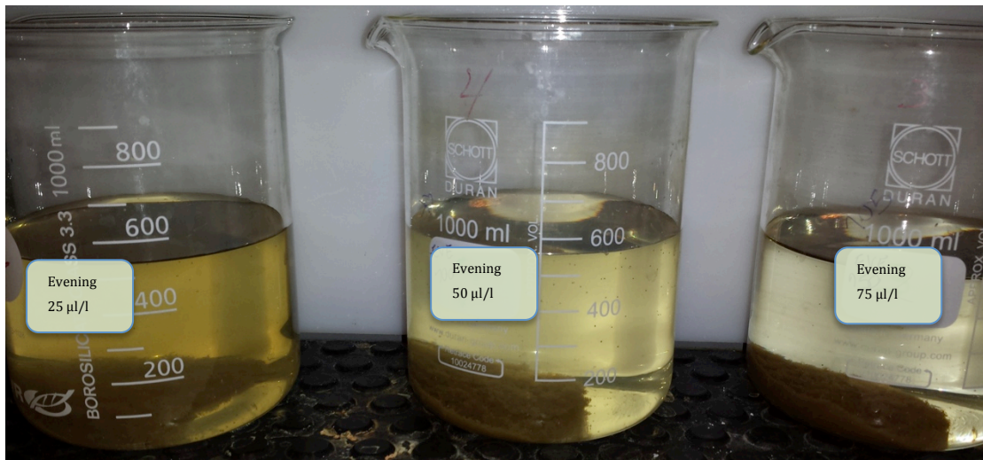
Figure 3-5 Evening water on the 19th of March with doses of 25, 50 and 75 microliters of JKL
