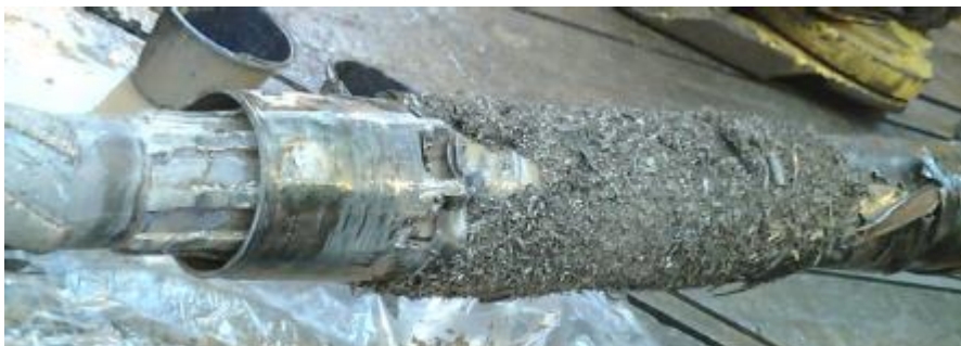
Figure 4.3.1 Casing retrieved to surface after milling operation, containing a swarf “birdsnest”
