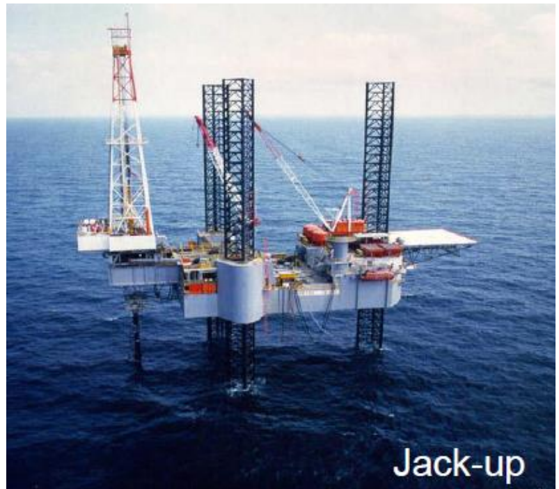
Figure 6.2.1. Typical jack-up rig with three legs. [14]
