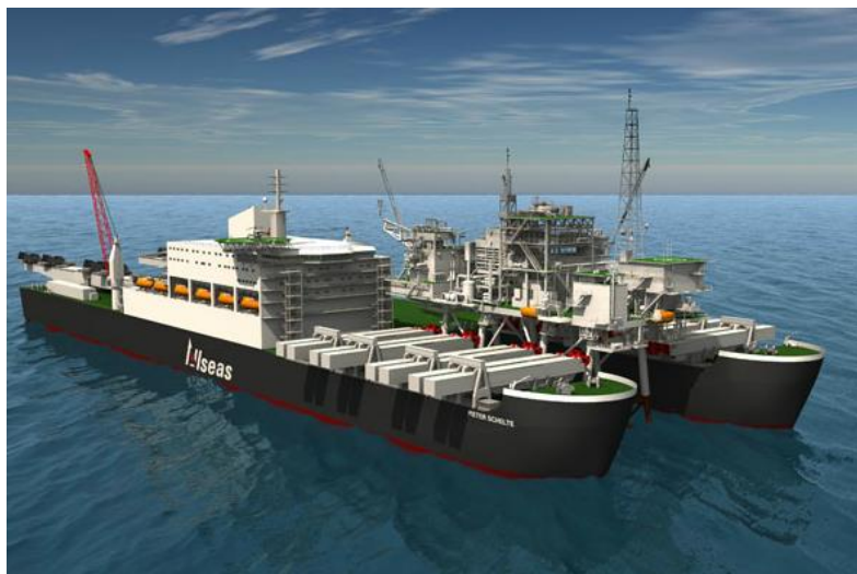
Figur 5.3.2.1 Pieter Schelte, specialized decommissioning vessel. [13]
