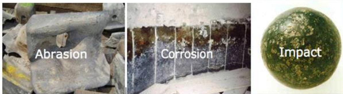
Figure 14 Wearing of some mill components such as balls and liners as a result abrasion, corrosion and impact (Source: Magotteaux, 2010)
