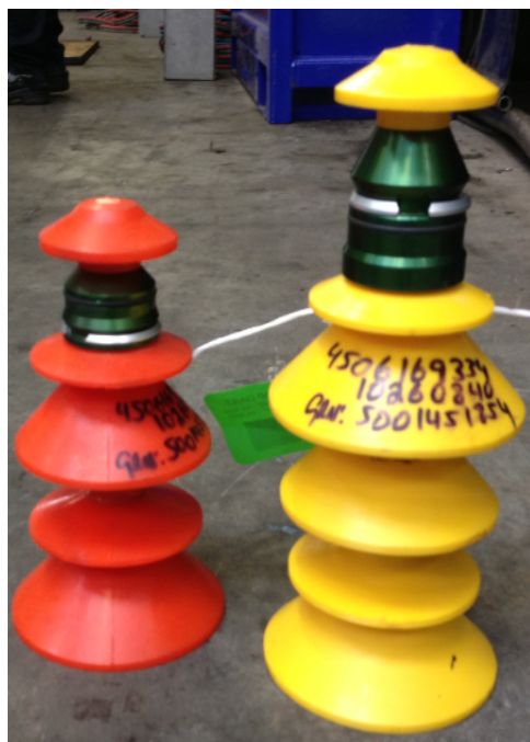
(a) Wiper darts installed in cement head. (b) Wiper plugs installed in liner hanger.
