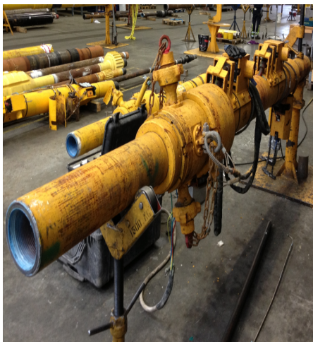
(a) Cement head used in well 2/8-G-3.
