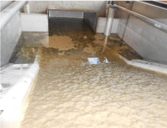
Figure 3-12: SF1000 biofilm flocs initial filtration (left) and during air knife cleaning (right)
