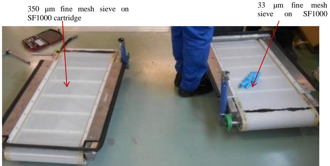
Figure 3-28: 350 and 33 \mu\text{m} fine mesh sieve on SF1000 cartridge
