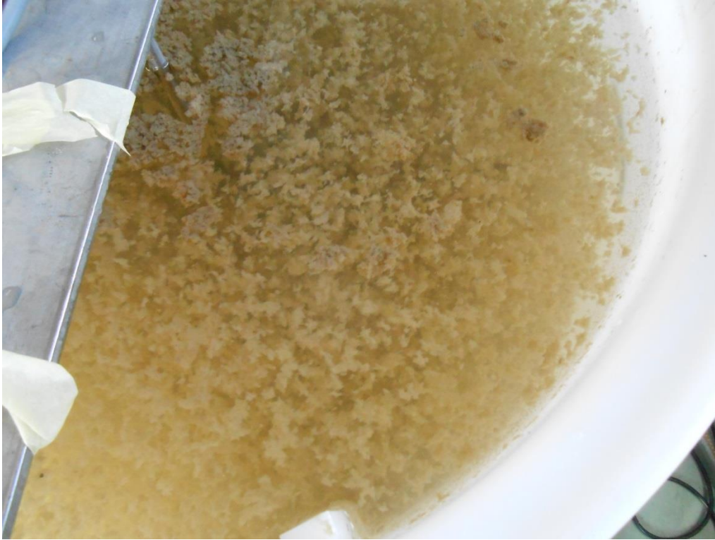
Figure 4-6: First trial of C-496 with PAX-18 doses at jar-test optimum parameters on pilot scale coagulation/flocculation tank.
