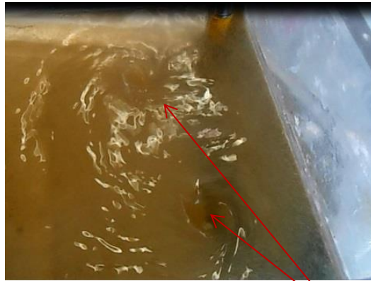
Shear current created due to the gap between the lower roller and the inner plate
