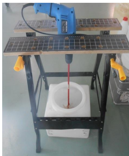
Figure 3-3: Polymer preparation setup at NFR wwtp
