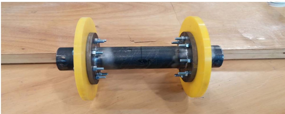
Figure 8.3: Shore grade 65 Pig
