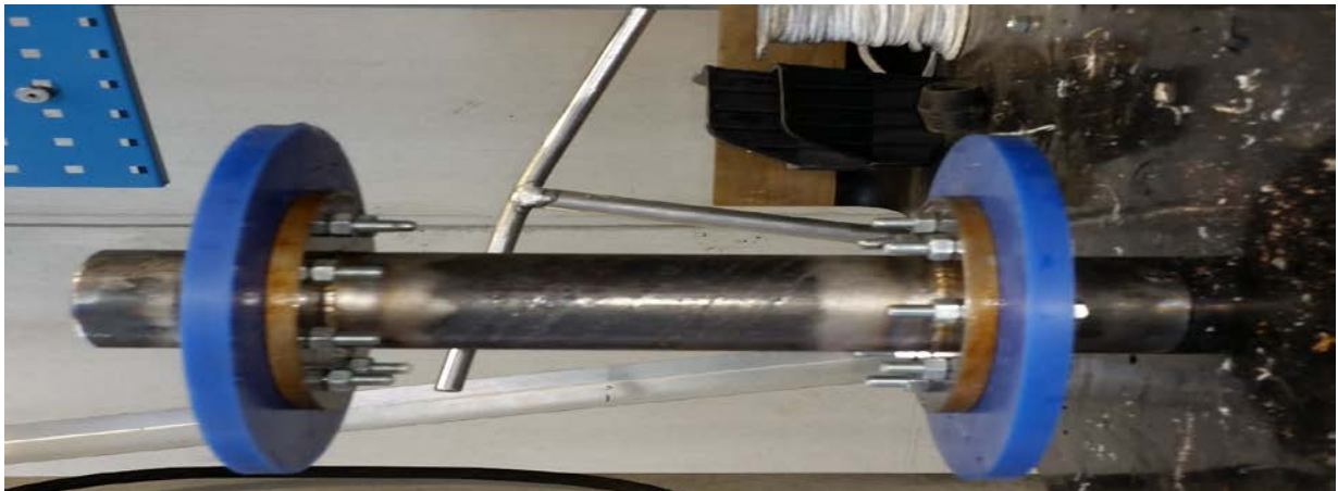
Figure 8.5: Shore grade 85 Pig
