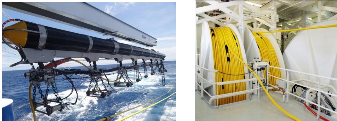
Figure 3 Source arrays and streamer winches
