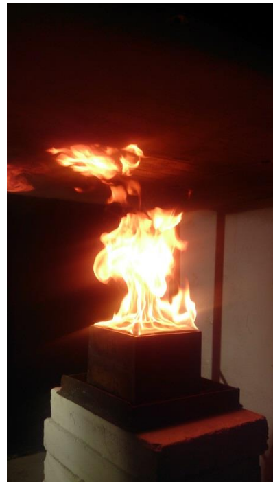
Figure 3 Picture of diffusion flame from experiments performed by Mats Flo on HSH
