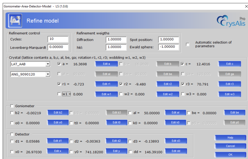
Figure 2.16: The Refine instrument model . In this example with a hexagonal lattice, the only free lattice parameters are a and c .
