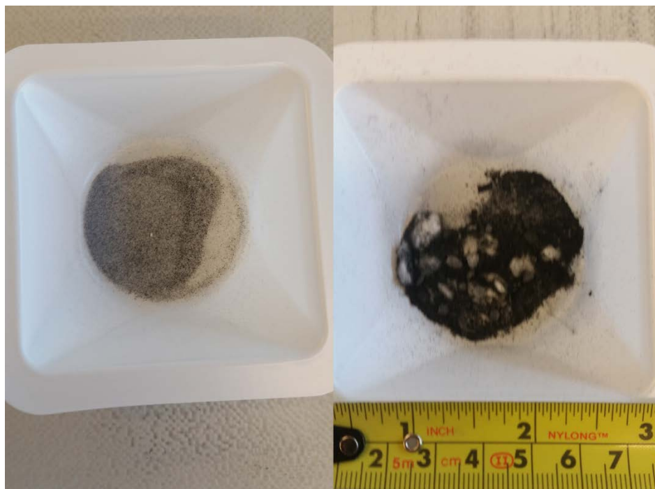
Figure 4.14: Left: Catalyst diluted in \gamma -Al 2 O 3 ; Right: fraction of deposited carbon in the small stainless steel tube and quartz wool plugs
