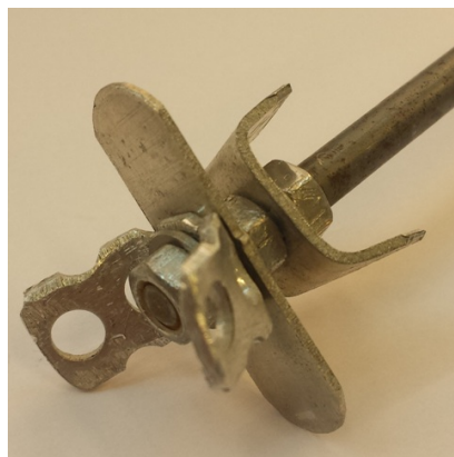
Figure 4.12: Mixing part of the turbine
