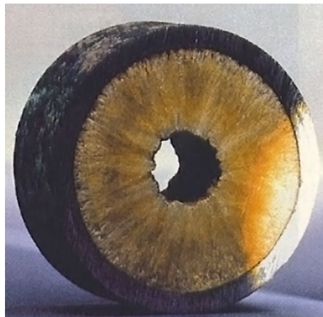
Figure 4: Wax deposition in a subsea pipeline [8]
