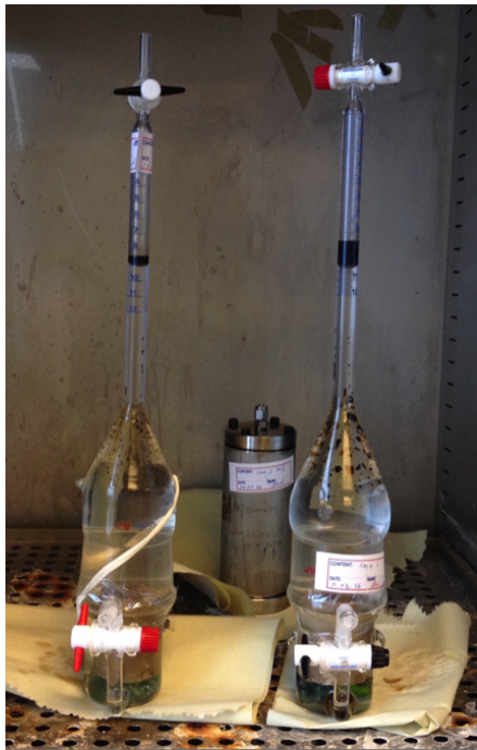
(a) two in front) Spontaneous imbibition of SK-10 and SK-0; and aging of SK-40 (back).
