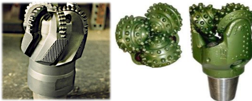
Figure 4: PDC bit with five blades (left) and roller cone bit (right) [5].
