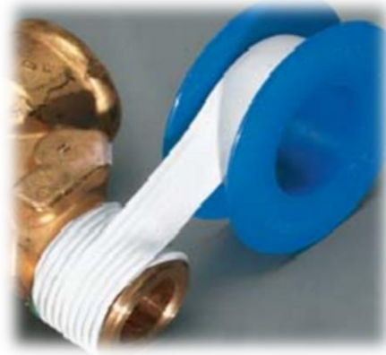
Figure 68: Thread taping to avoid leaking.
