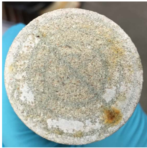
Figure 25. Filter cake in Berea sandstone core after injected with 0.14\ \mu\text{m} particle
