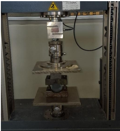
Figure 2.9 Zwick Z200 manufactured by Zwick GmbH Germany used to perform a Brazillian test
