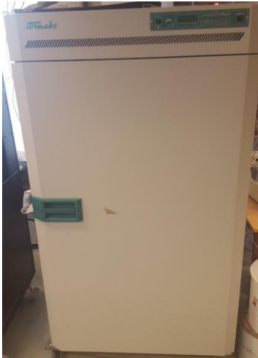
Figure 2.7 Oven used for curing the samples at the required bottom hole temperature.
