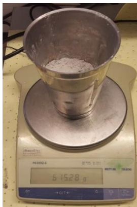
Figure 2.2 A Mettler Toledo mass balance that was used for accurately weighing the materials
