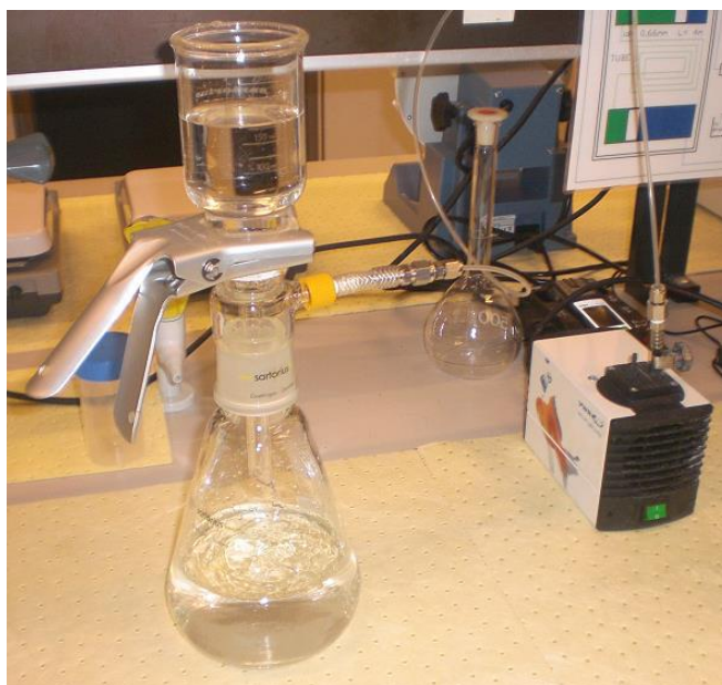
Figure 12: Brine Preparation: Filtration setup 27
