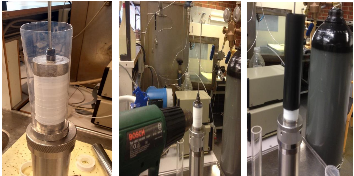
Figure 16: Core wrapping, Heating of plastic cover & putting rubber cover 27
