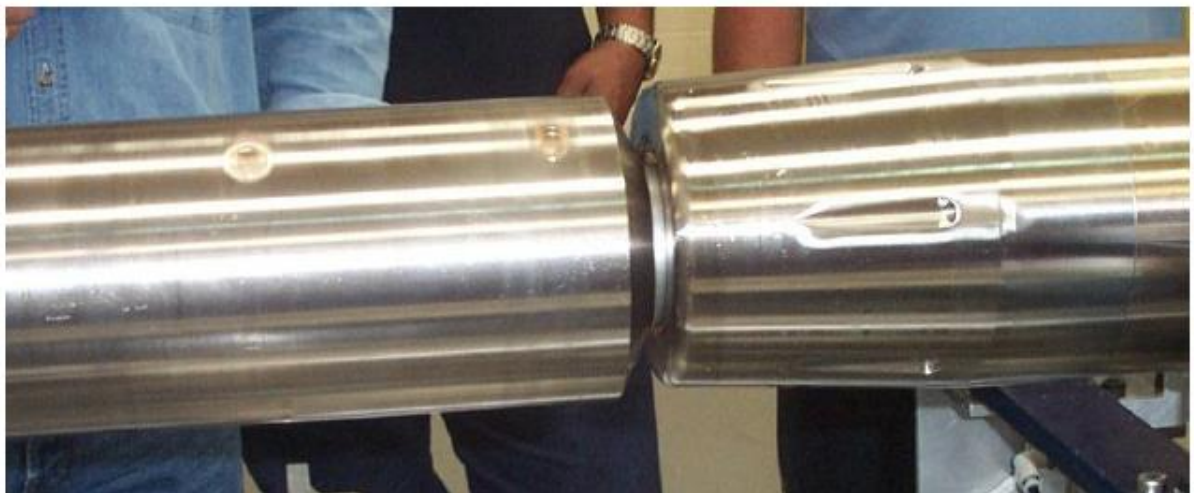
Figure 2.18. Deflection of RSS during testing
