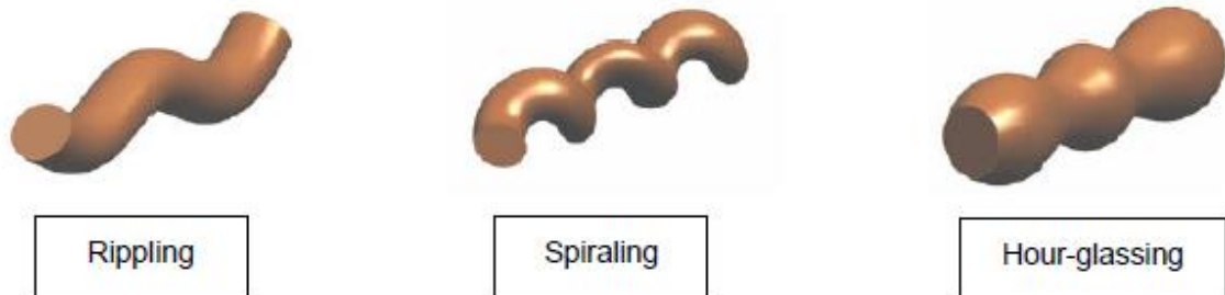
Figure 2.27. Different drill-sting stress conditions
