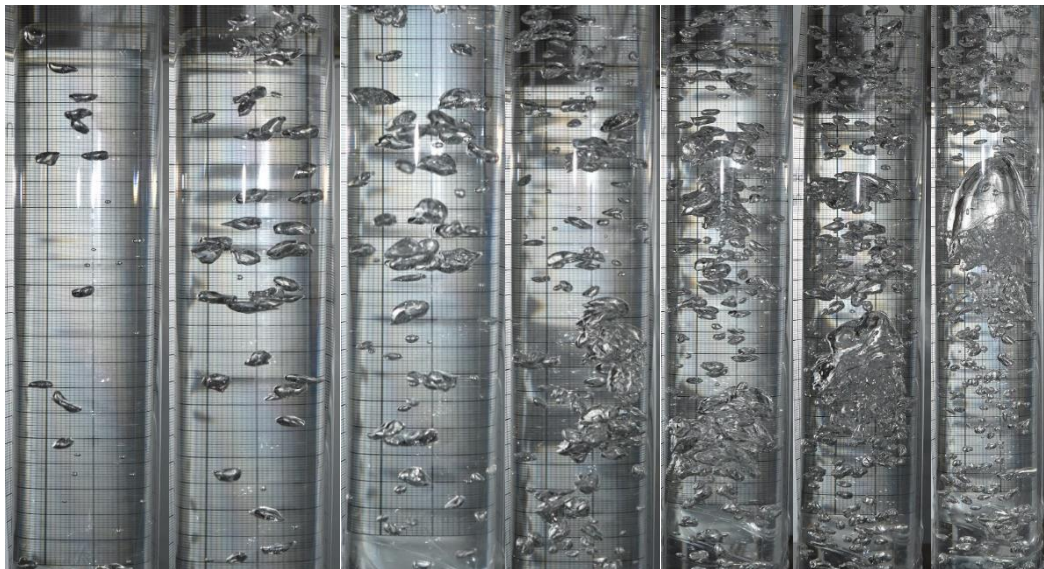
Figure 30- Flow pattern at 0,2; 0,5; 1,0; 1,5; 2,0; 2,5; 3,0 SPLM of gas (air) respectively
