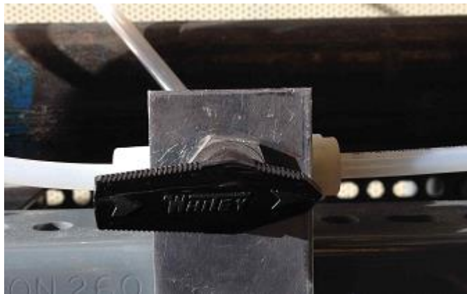
Figure 41- Valve 2 directing gas towards model
