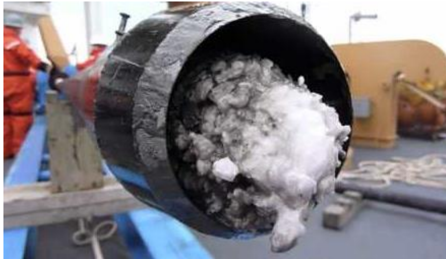
Figure 2-4 Gas methane hydrate recovered in core catcher during bottom sampling aboard USCGC Healy in the Southern Beaufort Sea in 2010 [34].
