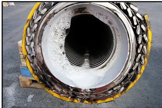
Fig. 2.1 Cross-section of flexible riser (Muren et al., 2013)
