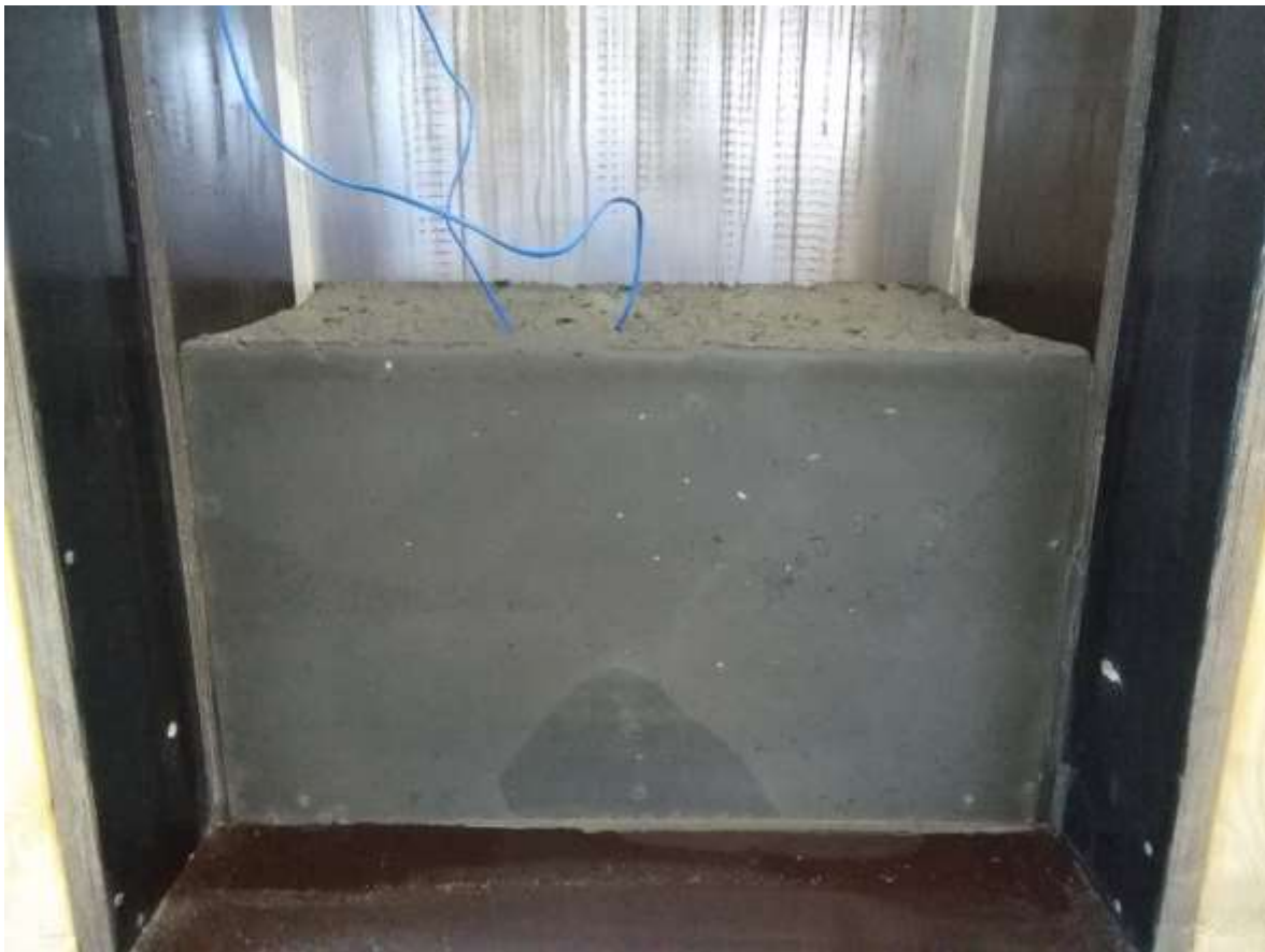
Figure 21 - Cured concrete block in the slipform rig
