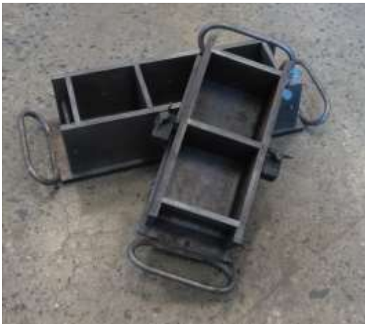
Figure 19 - Moulds for cubes
