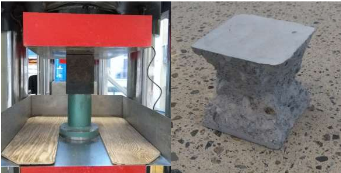
Figure 22 a/b - Testing of compression strength and tested cube
