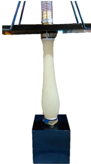
Figure 43. Balloon bulging at 100 per cent elongation and containing 0.7 litres of water
