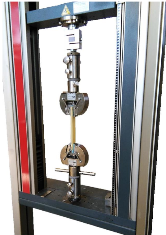
Figure 38. Balloon tensile test setup
