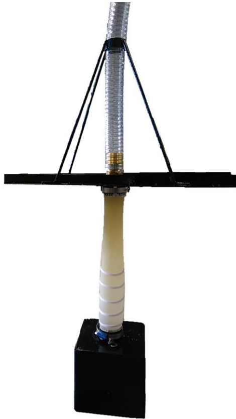
Figure 44. The prototype with the balloon circumferentially constrained with shoelaces
