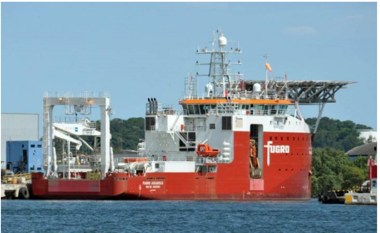
Figure 6. Typical ROV support vessel – Fugro Aquarius [34]
