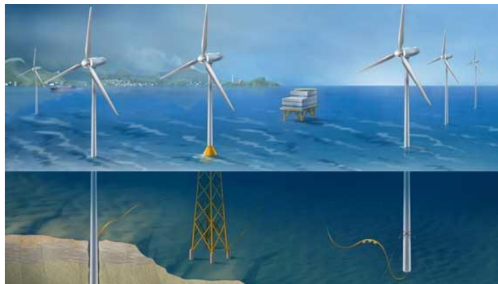
Figure 1.3: Fixed offshore wind turbine substructure concept [11]
