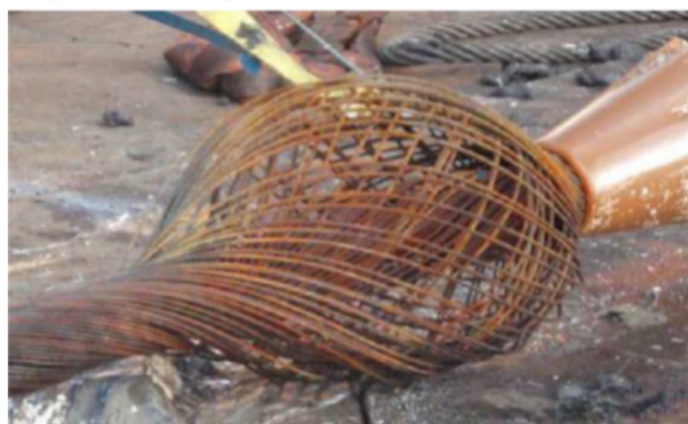
Figure 3-6: Picture showing a steel wire with a phenomenon called bird cage caused by twist in wire in addition to a sudden load change. [16]
