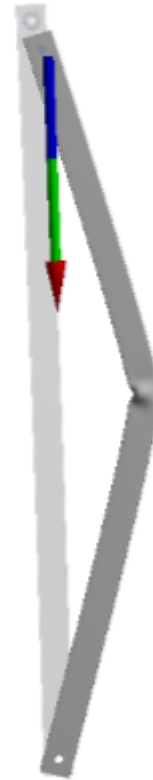
Figure 24: Buckling deformation, L = 5000 mm
