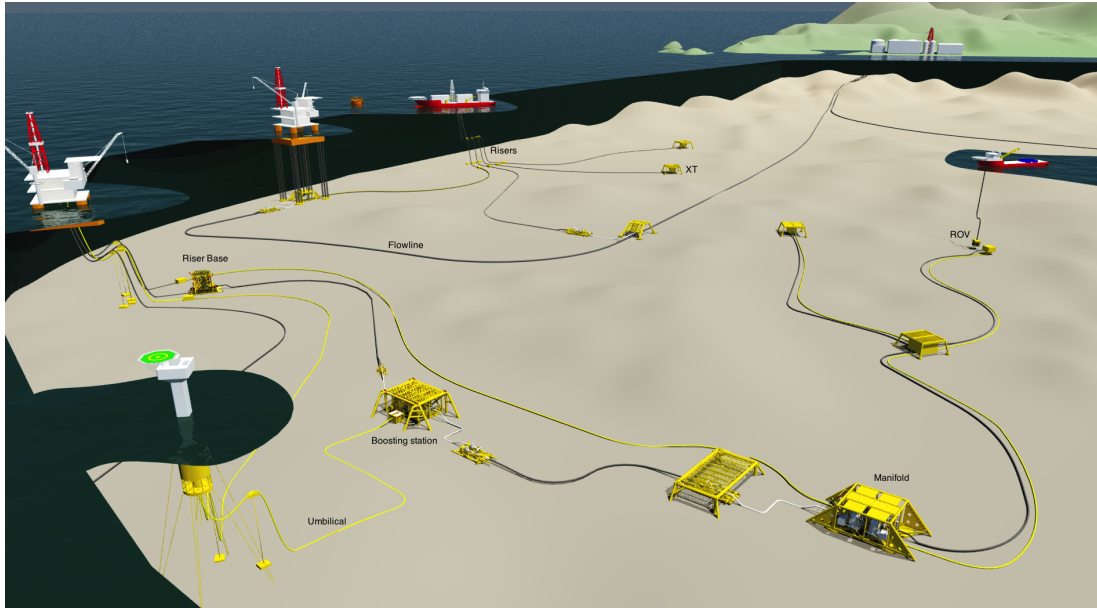
Figure 1: Typical subsea production system layout
