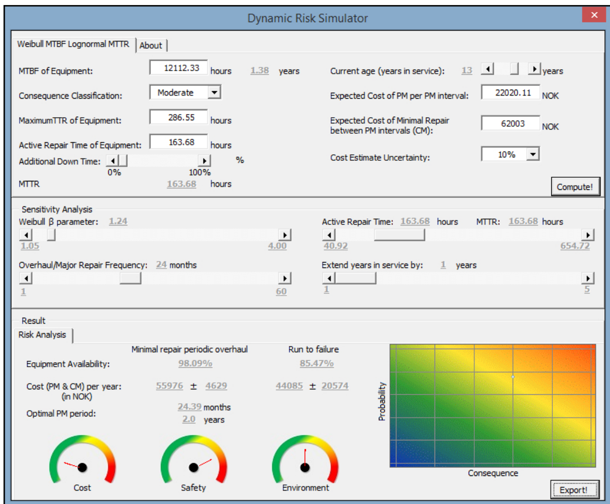
Figure 4.1: Screenshot of the Dynamic Risk Simulator with input data from the water injection booster pump
