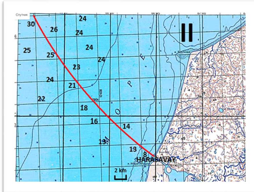
Figure 6.4. The pipeline route in the second section (shallow water) shown in the bathymetric map
