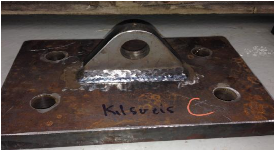
Figure 2.1 – the 3.25-ton pad eye [1]
