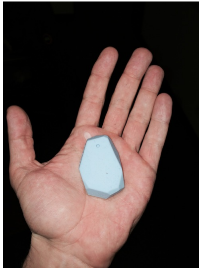
Figure 2.4: The size of an Estimote beacon compared to a hand. This is actually one of the bigger beacons on the market.
