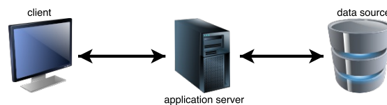
Figure 2.9: Three-Tier architecture: Client, server and data storage
