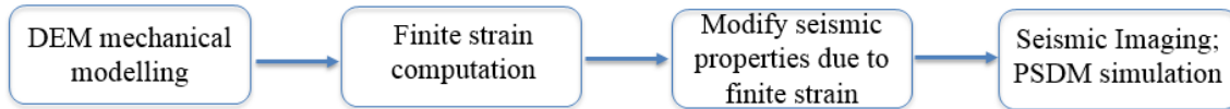
Figure 4: Methodology: From mechanical model (DEM) to seismic image. Workflow from Botter et al (2014).
