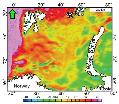
Figure 13: Bouguer map, with a reduction density of 2200kg/m<sup>3</sup> offshore and 2670kg/m<sup>3</sup> onshore. Modified from Marello (2012).
