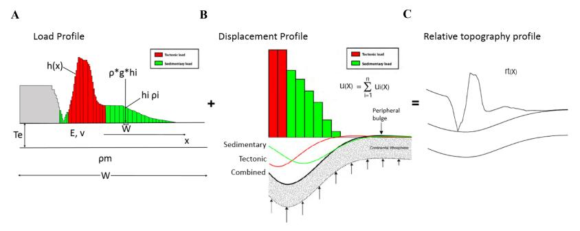
Figure 11: Example of how the load profile (A) and displacement profile (B) relates to tectonic and sedimentary loads and combines to form the relative topography profile (C) (Modified from Campos, 2011; Cardozo and Jordan, 2001).
