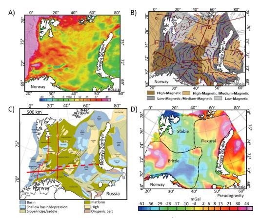
Figure 2: (A) Bouguer anomaly map (reference density =  $2260 \text{ g/m}^3$ ), (B) magnetic map with magnetic trends and fault zones, (C) map of the structures in the Barents Sea and (D) Pseudogravity map divided into three different zones due to their flexural behavior and analysis of map A, B and C. Modified from (Marello et al., 2010; Henriksen et al., 2011; Marello, 2012)
