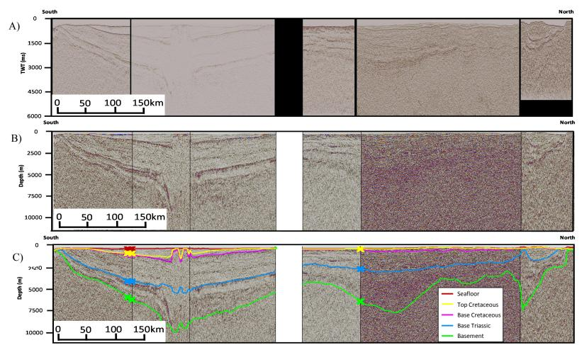
Figure 18: The eastern of the north-south trending transect lines, showing the seismic lines used in time (A), depth (B) and with interpretations (C). The vertical 26 exaggeration is set to 20 for both figures.
