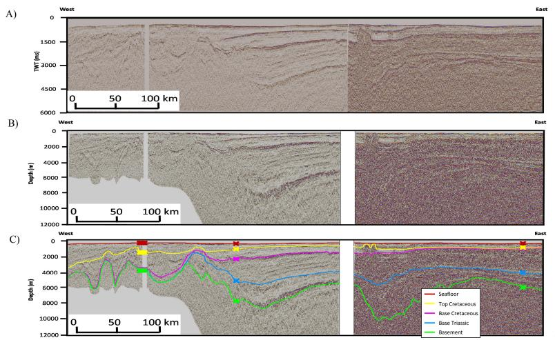
Figure 19: The east-west trending transect line, showing the seismic lines used in time (A), depth (B) and with interpretations (C). The vertical exaggeration is 27 set to 12.5 for both figures.
