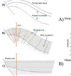
Figure 26: Flexural Slip unfolding principle. A shows the input beds and fault, B shows how the program uses bisectors and a given direction (pin) to restore the transects into C.
