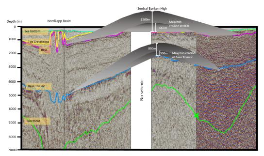
Figure 28: Example showing the amount of minimum and maximum erosion that was calculated in Sentral Banken High for sequence two and three.
