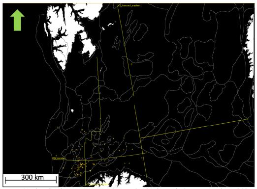
Figure 16: The yellow lines are 2D seismic lines used in this thesis. The Seismic was only available in the Norwegian sector. The white contours are the different structures found in the Barents Sea. The wells with time depth relationship is marked in orange and is mainly located south.
