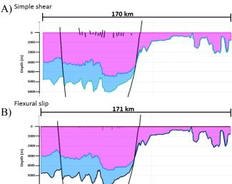
Figure 27: Simple shear (A) versus flexural shear (B) for a seismic line crossing the Hammerfest Basin.
