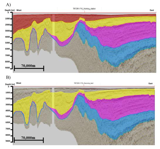
Figure 25: (A) Before decompaction and (B) after decompaction. The sequences in figure B thickened due to the decompaction process and were used as an input for the restoration part. The vertical exaggeration is 15 times in both figures.
