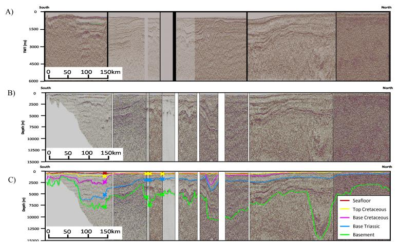
Figure 17: The western of the north-south trending transect lines, showing the seismic lines used in time (A), depth (B) and with interpretations (C). The vertical exaggeration is set to 15 for all figures.
