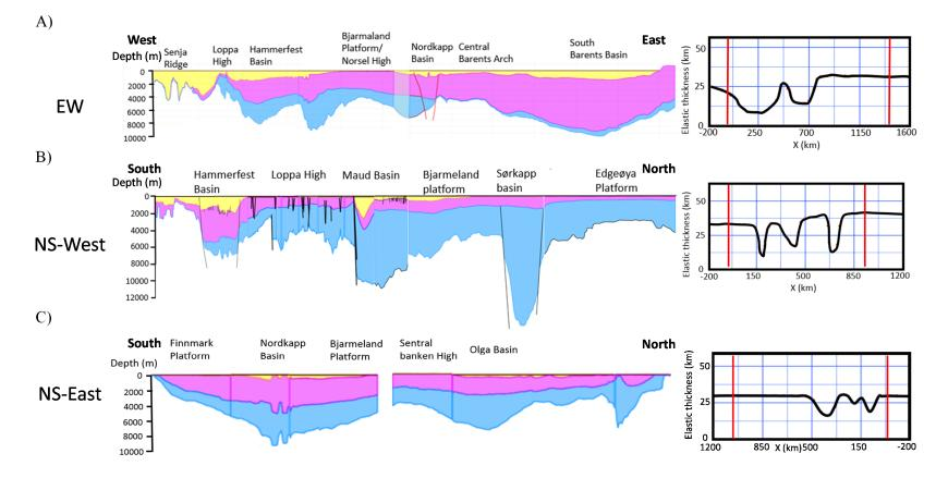
Figure 29: Example of the three transect lines (here restored at top cretaceous). To the right, between the red lines, are the same transects showing the variation in elastic thickness throughout the transect lines. The transect lines shown are (A) the east-west trending, (B) the western north-south trending and (C) the eastern north-south trending transects.
