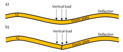
Figure 12: Example of a continuous (a) and broken (b) elastic plate with the vertical loads applied and deflection due to the tectonic and sedimentary loads.
