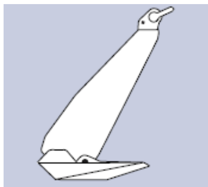
Fig 1.2: Drag embedment anchor (Source: Vryhof anchors)
