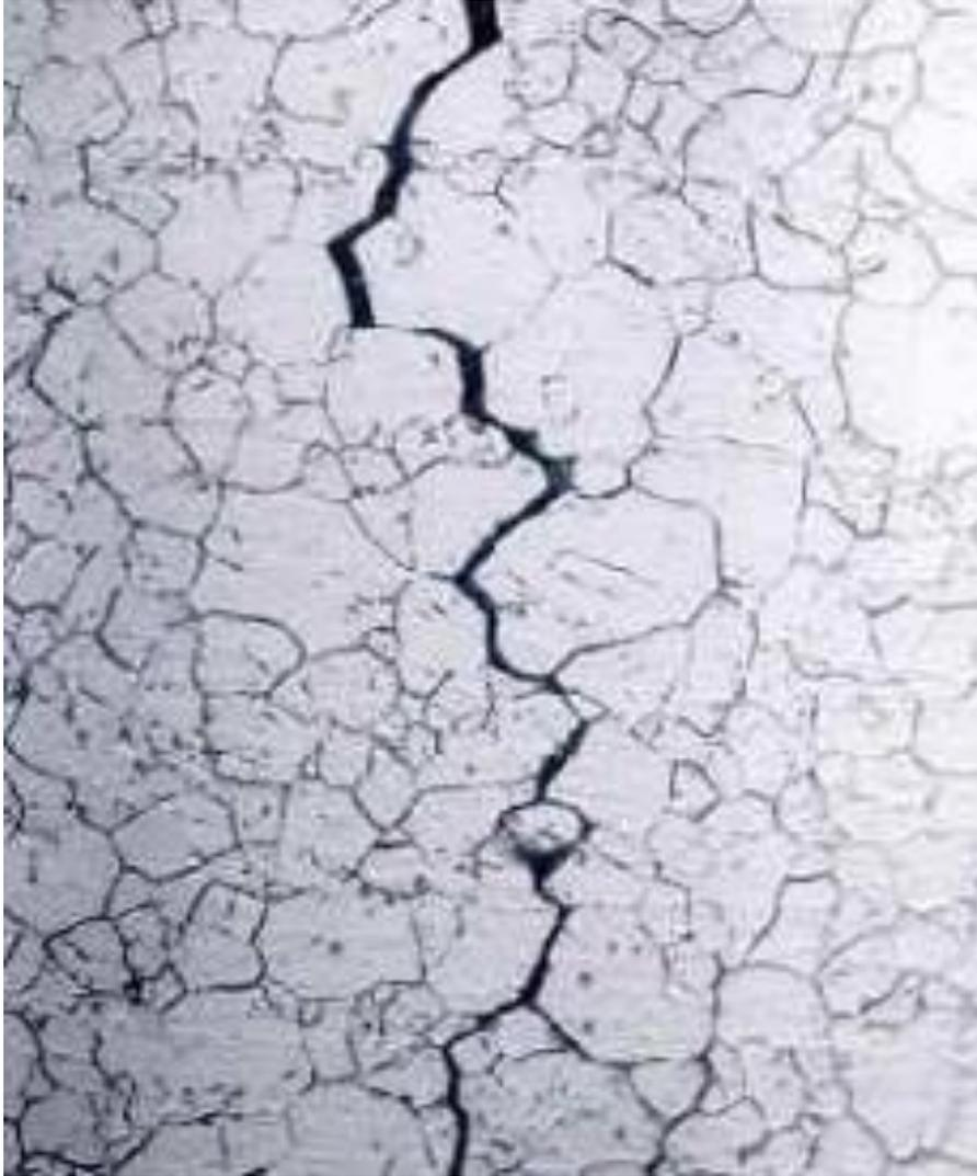
Figure 2.14: Intergranular stress corrosion cracking (NACE international, n.d)
