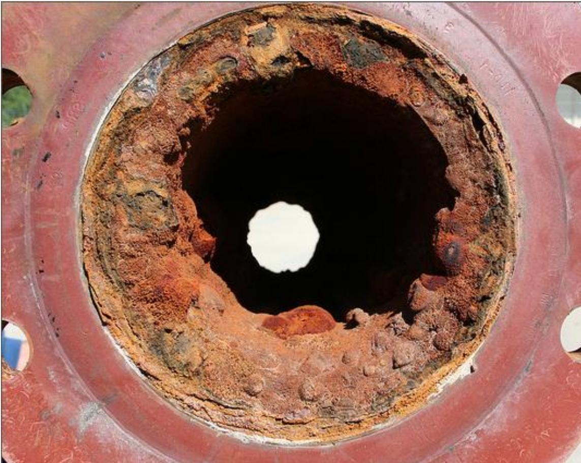
Figure 2.12: Internal CO<sub>2</sub> corrosion. (Liberty corrosion, n.d)
