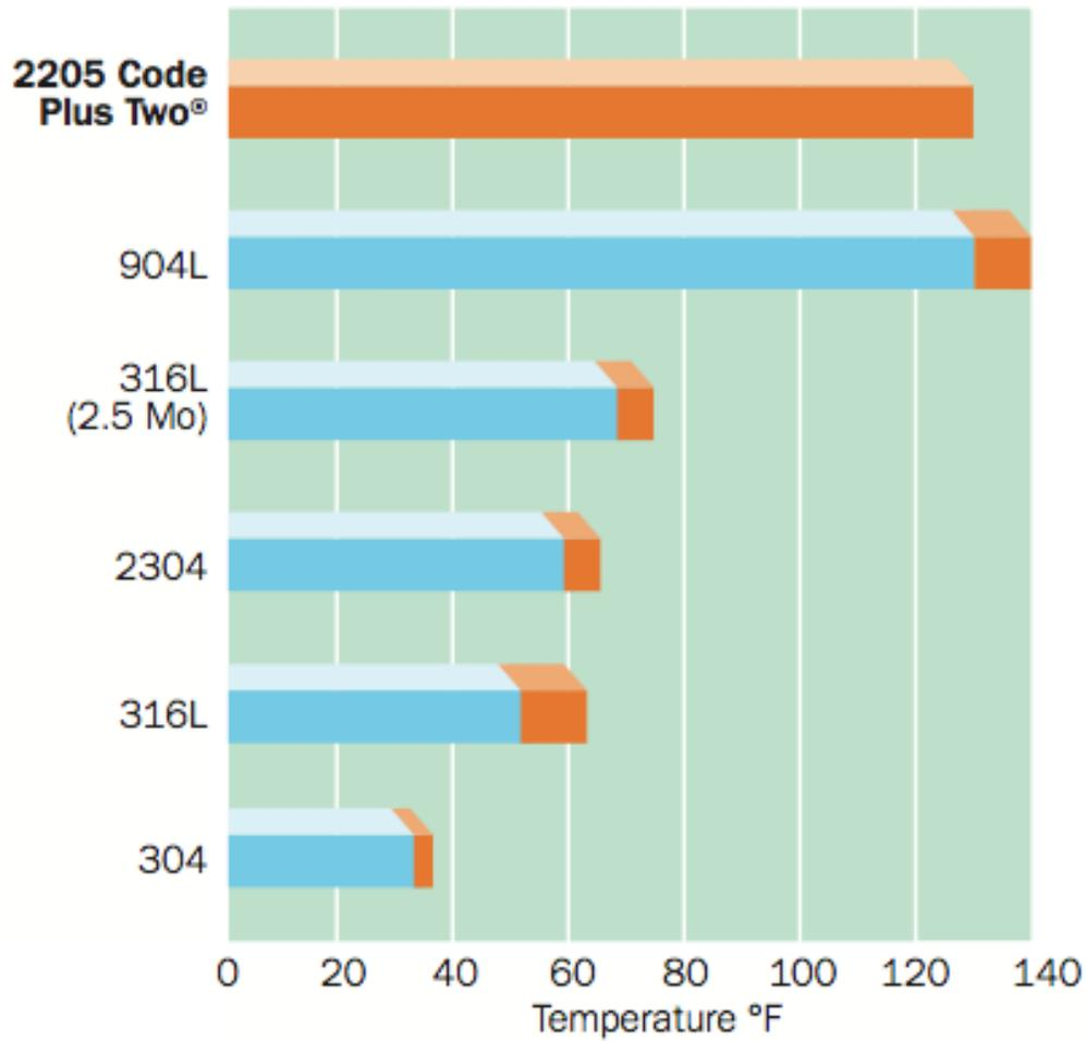
Figure 2.7: Critical pitting temperature in NaCl. (Outokumpo, n.d)
