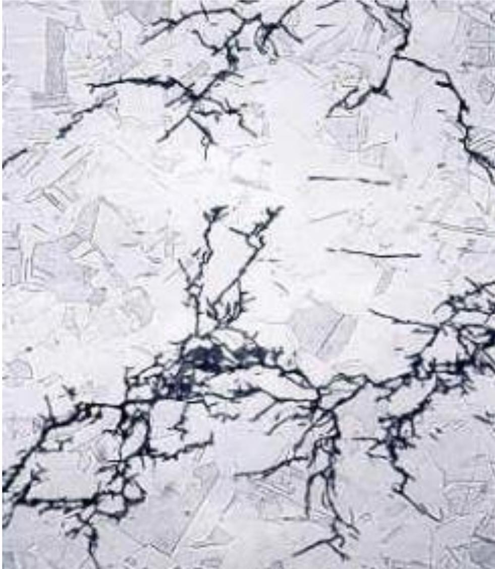
Figure 2.15: SCC in a 316 stainless steel chemical processing pipe.
