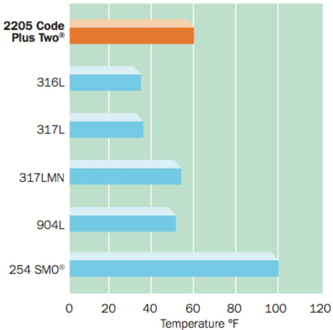
Figure 2.8: Critical crevice corrosion temperature (Outukumpu, n.d.)
