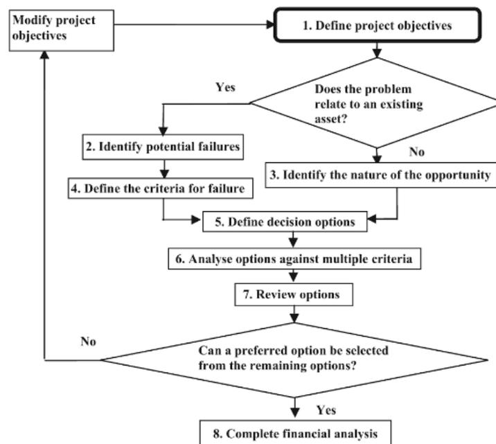
Figure 3: FMAD: Flexible Asset Maintenance Decision-Making Process Based on NAMS (Amadi-Echendu et al., 2012)
