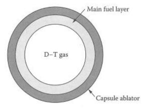
Figure 34 Schematic picture of target capsule (Pfalzner, 2006, p. 14).
