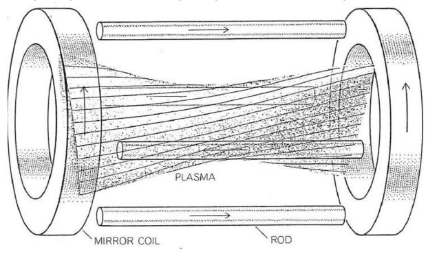
Figure 10 Simple setup of a magnetic well. The resultant field (color) is twisted and increases in all directions from the center. The arrows shows the direction of the current (Fowler & Post, 1966, p. 26).
