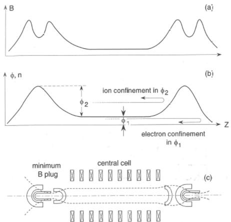
Figure 29 Principle of tandem mirrors. (a) Magnetic field on axis. (b) Plasma density potential on axis. (c) Coils for axisymmetric central cell and end plugs (Braams & Stott, 2002, p. 69).
