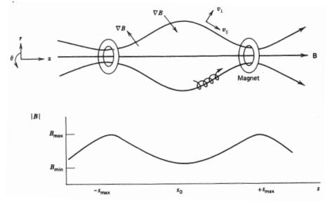
Figure 7 Simple mirror configurations (Stacey, 2010, p. 38).
