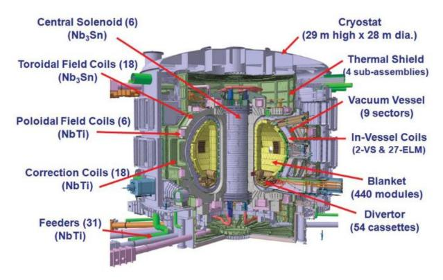
Figure 50 Schematic diagram of some of the component in ITER. Pay attention to the human in the lower right corner to as a reference for the size (Authority, 2014).
