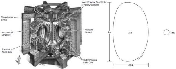
Figure 37 To the left a drawing of the JET design. To the right a comparison between JET and TFR (J Wesson, 1999, pp. 23,29).
