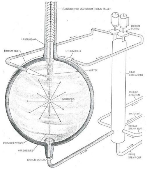
Figure 25 A proposed fusion reactor using laser and a frozen pellet of fuel (Lubin & Fraas, 1971, p. 28).
