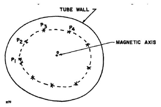
Figure 12 Cross section of stellarator tube. The points represents successive intersections of a single magnetic field line (Spitzer, 1958, p. 182).
