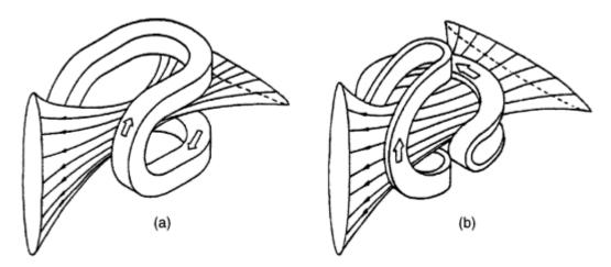
Figure 21 a) a "baseball seam" coil, b) a yin-yang coil set (Braams & Stott, 2002, p. 64).
