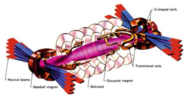
Figure 28 Schematics of Tandem Mirror Experiment, TMX (Dean, 2013, p. 55).
