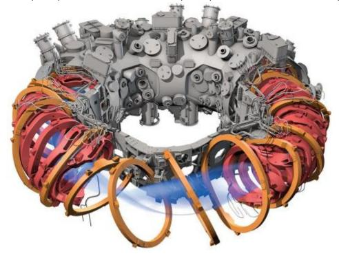
Figure 48 Schematics of the Wendelstein 7-X. The blue shows the plasma, the red rings are superconducting coils making the magnetic cage for the plasma and the orange rings are superconducting coils making fine adjustments to the magnetic field (Clery, 2015).
