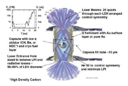
Figure 54 The indirect drive of NIF. Also shown is the laser pulse shape and hohlraum radiation temperature reached (Lindl, Landen, Edwards, & Moses, 2014).
