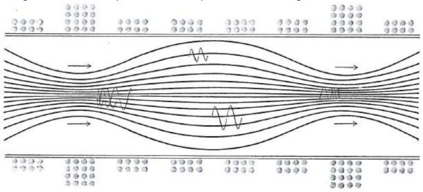
Figure 6 The magnetic mirror setup with magnetic field lines shown (Fowler & Post, 1966, p. 25).
