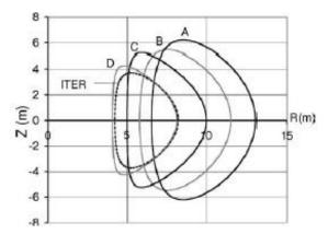
Figure 57 The size and shapes of the different PPCS models, with ITER as a reference (Maisonnier et al., 2005, p. 1175).
