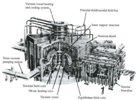
Figure 40 Overview of the most important parts of the TFTR machine (John Wesson, 2011, p. 637).
