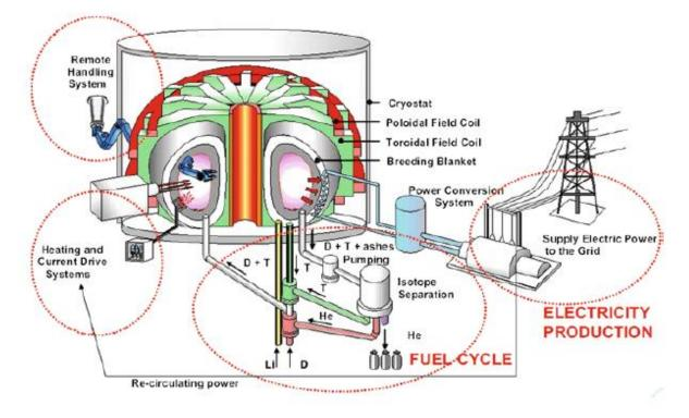
Figure 56 A Schematic of how researchers believes the main parts of a fusion power plant will be (F. F. Chen, 2011, p. 351).
