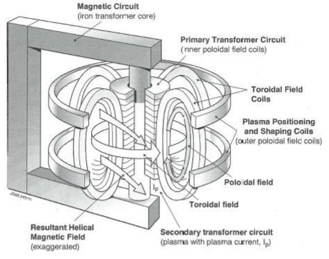
Figure 17 Schematics of a tokamak (Braams & Stott, 2002, p. 132).
