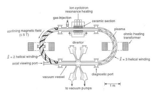
Figure 22 A simplified plan view of the C-stellarator showing major components (Braams & Stott, 2002, p. 125).
