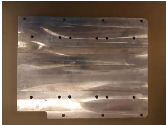
Figure 5.3: Water block IGBT mounting side
