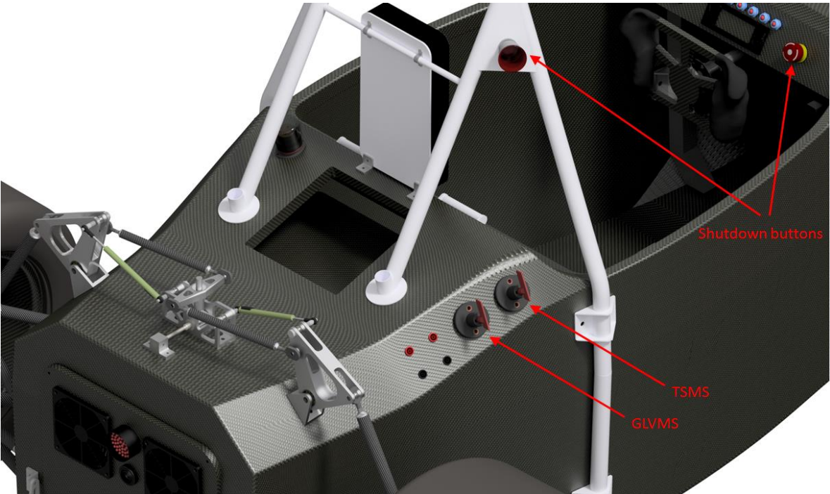
Figure 2.2 Shutdown circuit buttons outside group1 - Position
