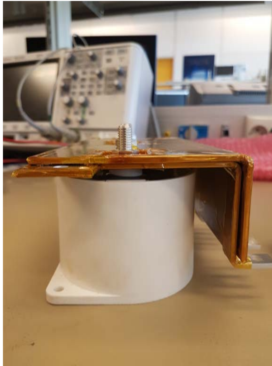
Figure 5.2: Busbar with added Kapton tape
