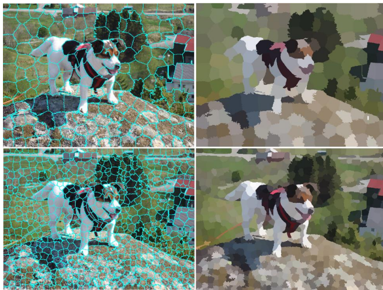
Figure 19: Example of a 960x720-image segmented into 200 and 800 superpixels, then put together based on the mean in each superpixel resulting in a more primitive description of the image. Notice how the superpixel edges adapt to the pixel regions and how the choice of the number of superpixel plays in the resulting segmentation.
