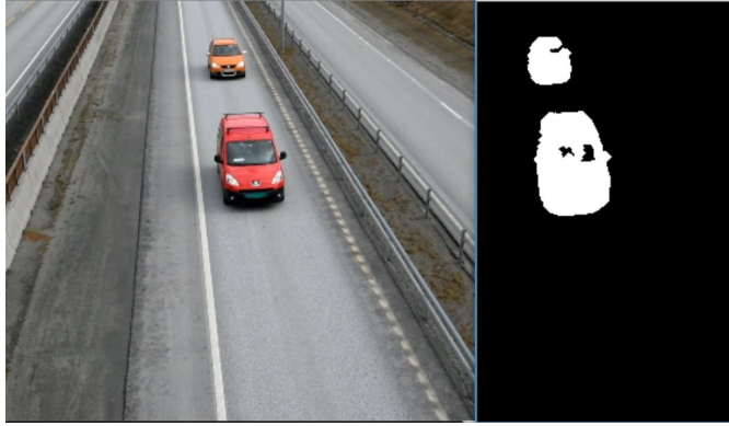
Figure 2.2: Extract foreground based on movement in the background image
