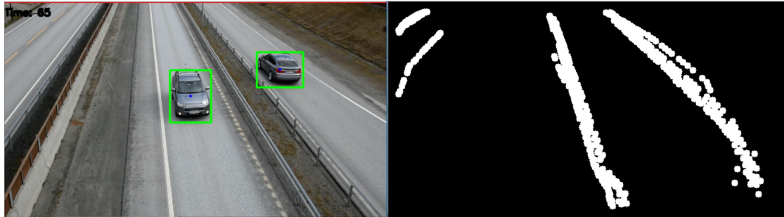
Figure 3.14: The lanes becomes apparent by tracking the movement in the foreground mask
