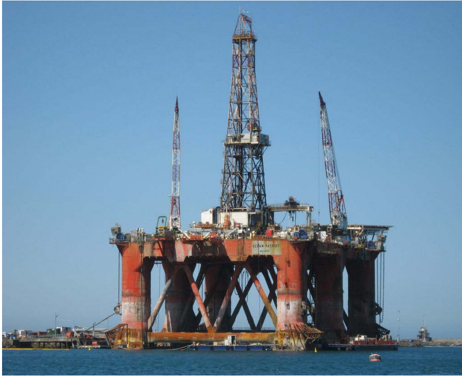
Figure A- 3: Ocean Patriot, a 3rd generation Bingo 3000 semisubmersible, built in 1983. Source; Kaiser et al., (2013)
