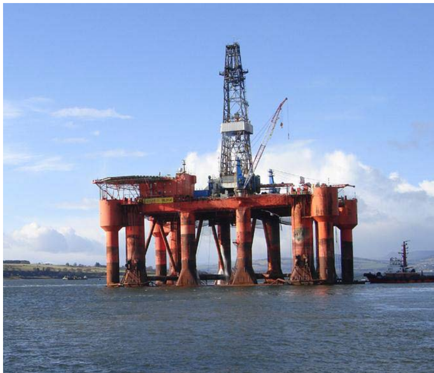
Figure A- 2; Essar Wildcat. A 2nd generation Aker H-3 submersible developed in 1977. Source; Kaiser et al., (2013)
