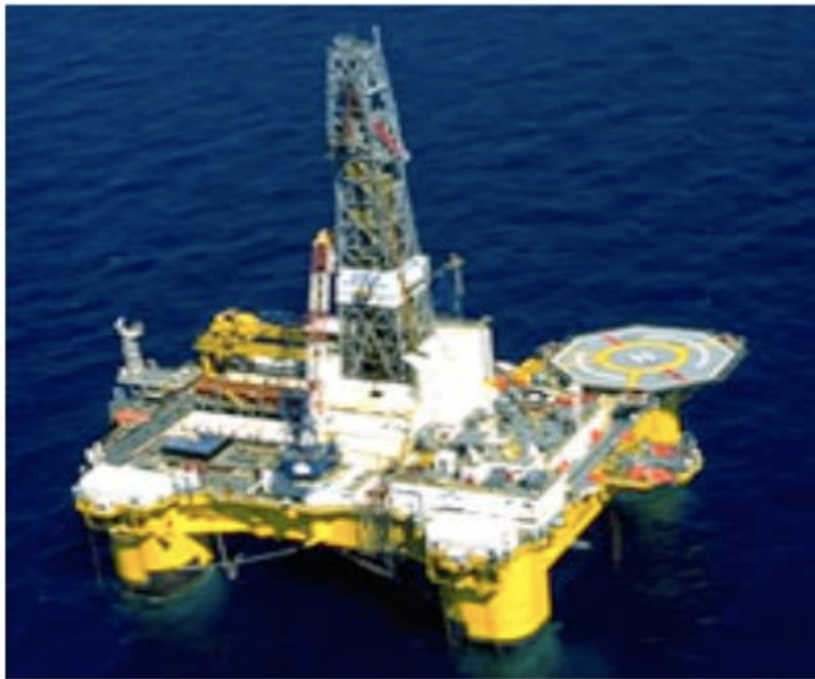
Figure A- 4; Transocean Richardson, a 4th generation semi-submersible, built in 1988/1991. Source; Deepwater, (n.d ,a)
