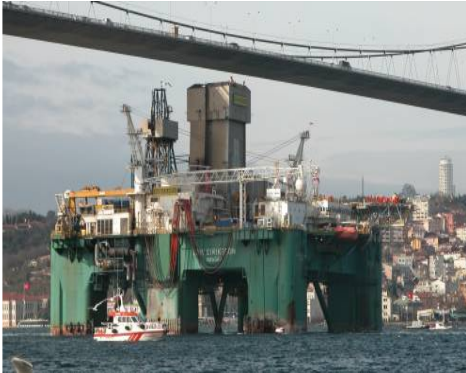
Figure A- 5; Leiv Eirikssen, a 5th generation semisubmersible, built in 2001. Source; Ocean Rig (n.d)
