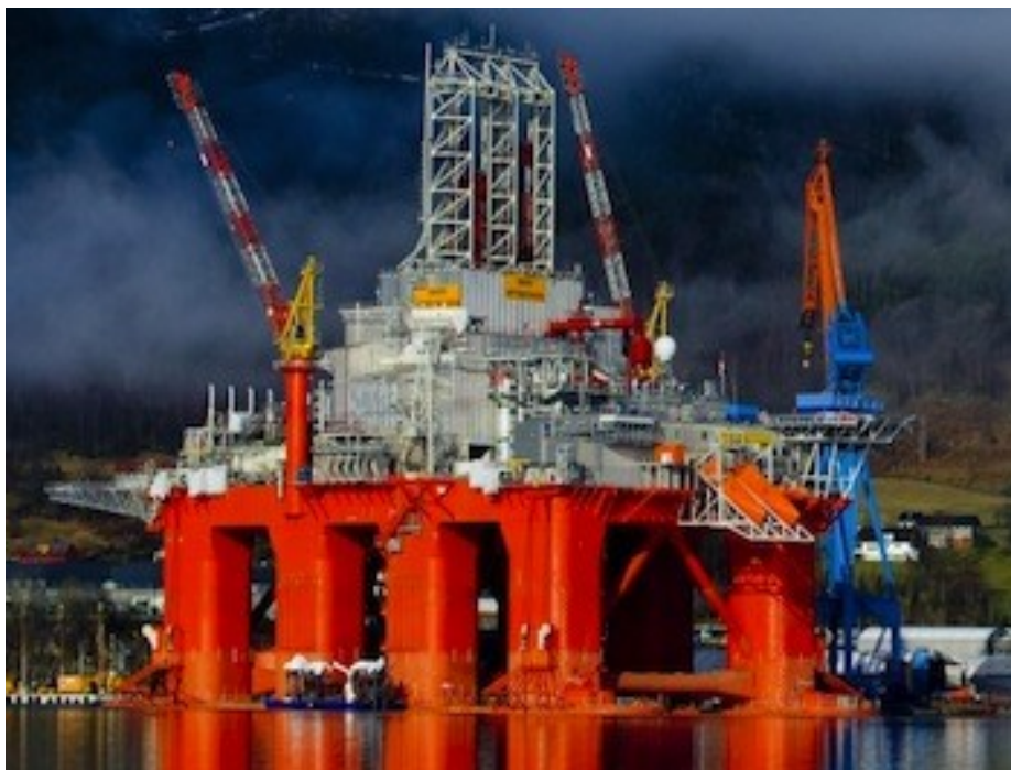
Figure A- 6; Transocean Spitsbergen a 6th generation semisubmersible Aker H-6e Semi-submersible , built in 2009. Source; Deepwater, (n.d ,b)
