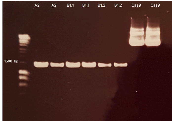
Figure 3.9: Samples from A2, B1 and Cas9 before digestion of plasmid. Bands from samples A2 and B1 were approximately 1700 bp, while Cas9 had several bands.
