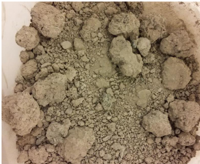
Figure 44: Structure of dewatered cuttings
