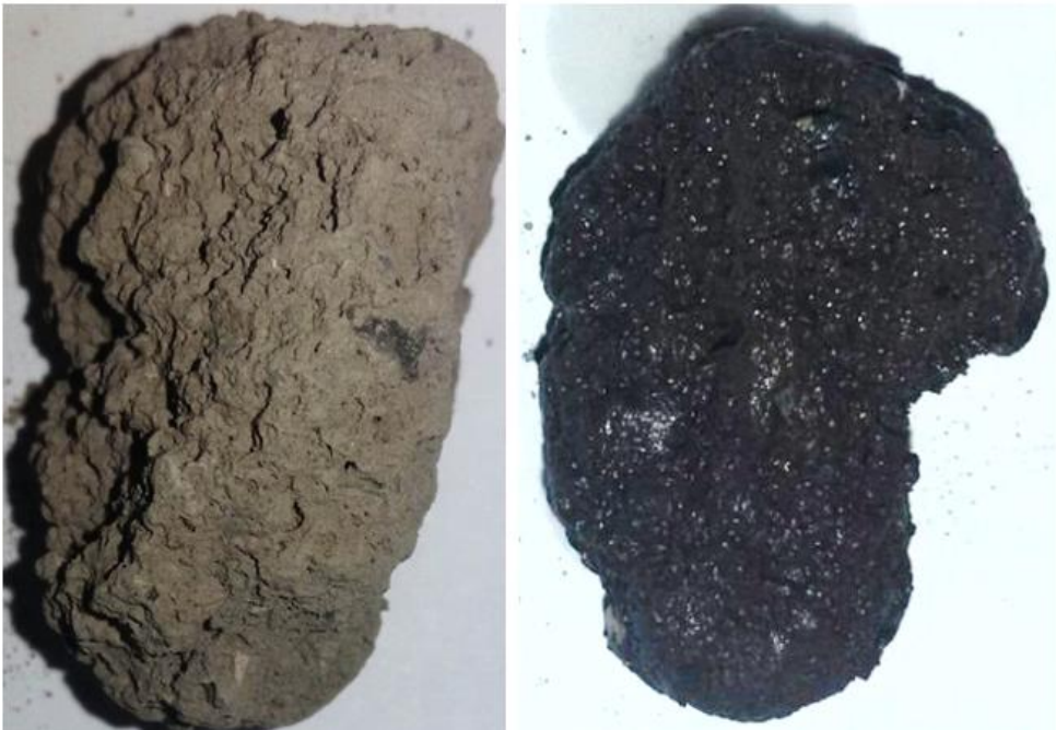
Figure 46: Dry sample on the left and sample doused with MEG on the right
