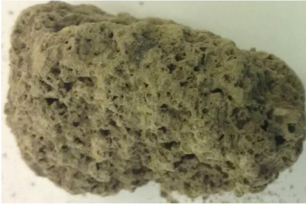
Figure 45: Dewatered cuttings showing pours
