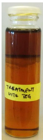
Figure 38: Decomposition of TEG on drill cuttings
