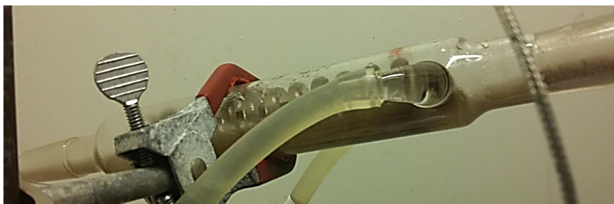
Figure 49: Condenser with solids entrainment
