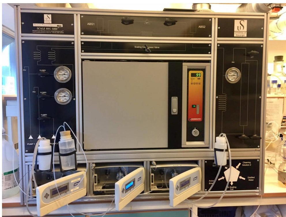
Figure 34 The scale Rig used for high-pressure tube blocking testing of SIs. (From the left: Pump 1, Pump 2, Pump 3)
