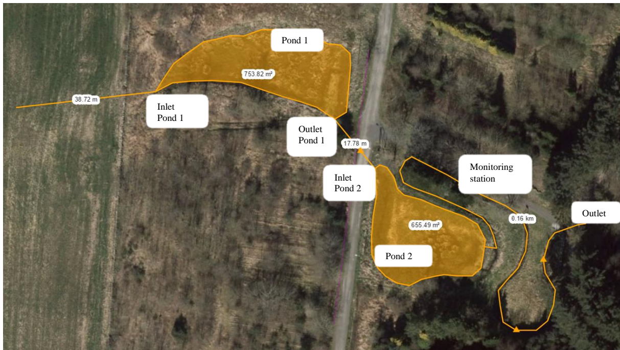
Figure 3. 3. Illustration of pond 1 and 2, which constitute the constructed wetland together with areal dimensions and important terms.
