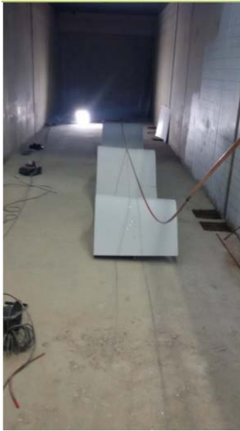
Figure 6-19: Residual Curvature in Sag configuration before Test is performed
