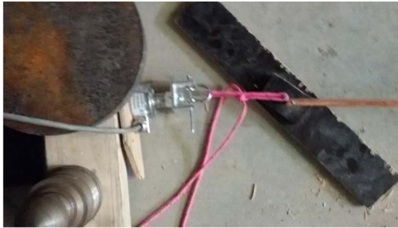
Figure 4-23: Load Cell Firmly Secured
