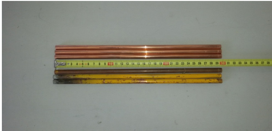
Figure 4-3: 300mm length of the old and New Pipe Pieces
