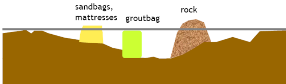
Figure 3-10: Pipeline Free Span Mitigation Measures (Karunakaran, 2015)
