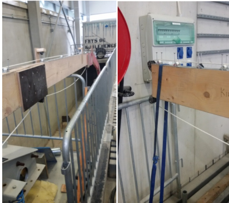
Figure 4-11: Applied Tension Pulley System on Stinger
