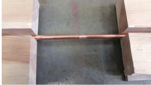
Figure 4-6: Pipe Connection with 8mm Diameter Pipe Inserted
