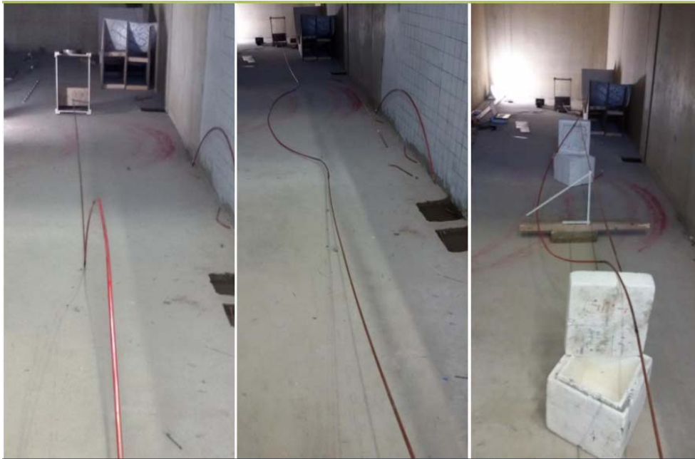
Figure 6-18: Pipe Rotation with a 3m R.C of 0.40% Residual Strain and 2-spring Pipeline Bottom Condition
