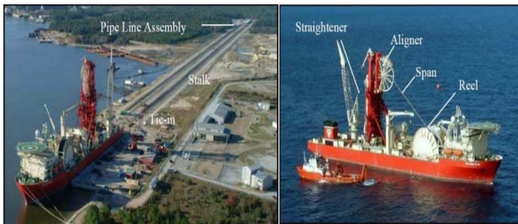
Figure 2-8: Reel Lay installation Vessel (Denniel, 2009)
