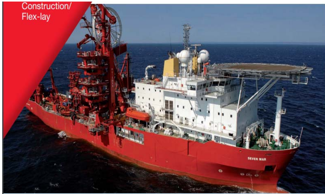
Figure 2-6: J-lay installation Vessel (Courtesy of Subsea7)
