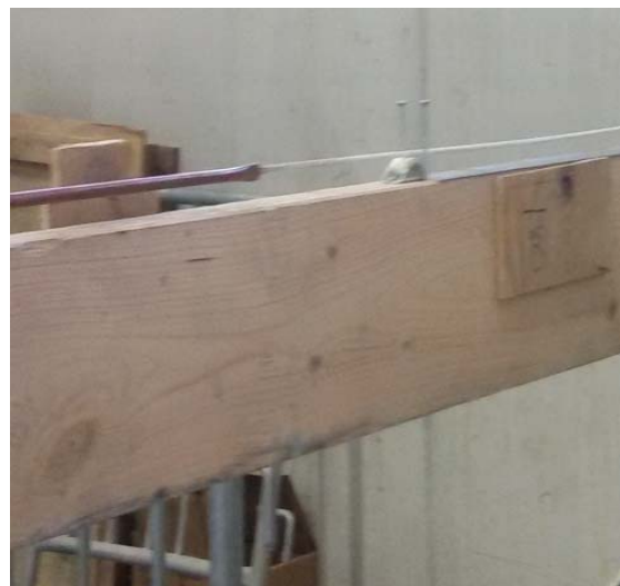
Figure 4-16: Pipeline End on Stinger Connected to Pulley System via String
