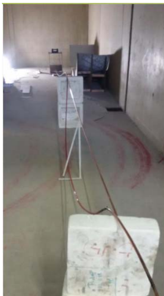
Figure 6-12: Pipe Rotation with a 3m R.C of 0.35% Residual Strain and 1-spring Pipeline Bottom Condition
