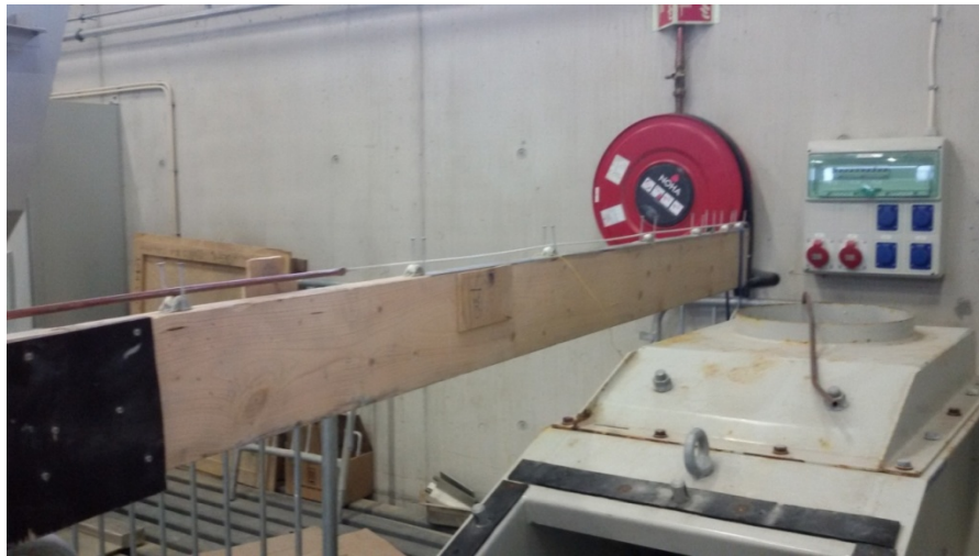
Figure 4-9: Rollers Placed on Stinger at Interval
