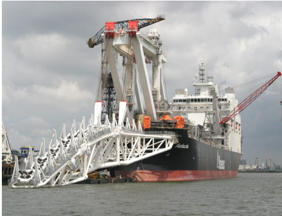
Figure 2-4: S-lay installation Vessel (Courtesy of Allseas Group)
