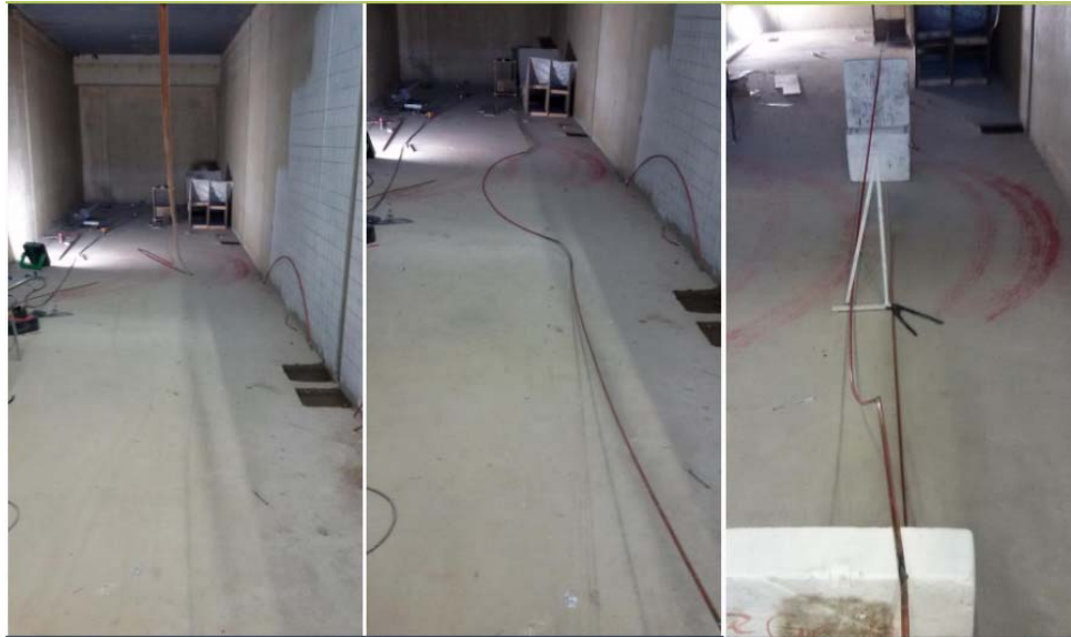
Figure 6-13: Pipe Rotation with a 3m R.C of 0.40% Residual Strain and 1-spring Pipeline Bottom Condition
