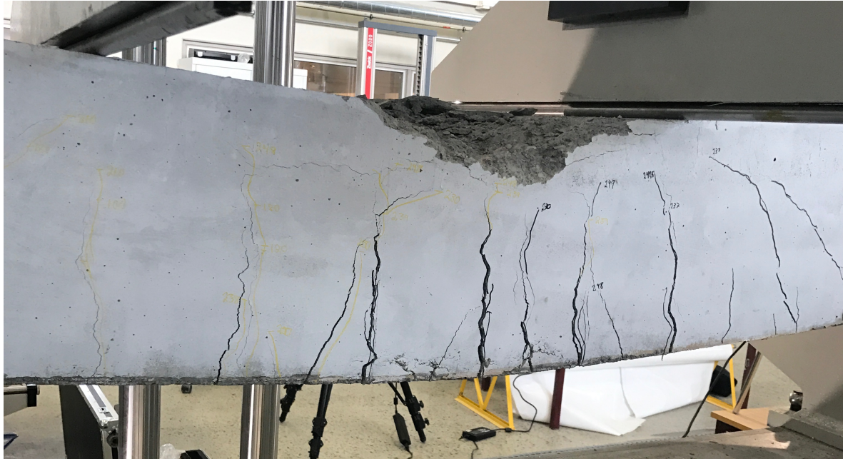
Figure 7-8: Crack pattern for reference beam at laboratory at a displacement of 53mm
