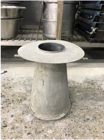
Figure 5-4: Slump flow measure of 0.5% RFRC sample.
