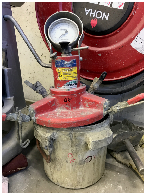
Figure 5-2: Equipment for measuring the air content and the density of the concrete samples.
