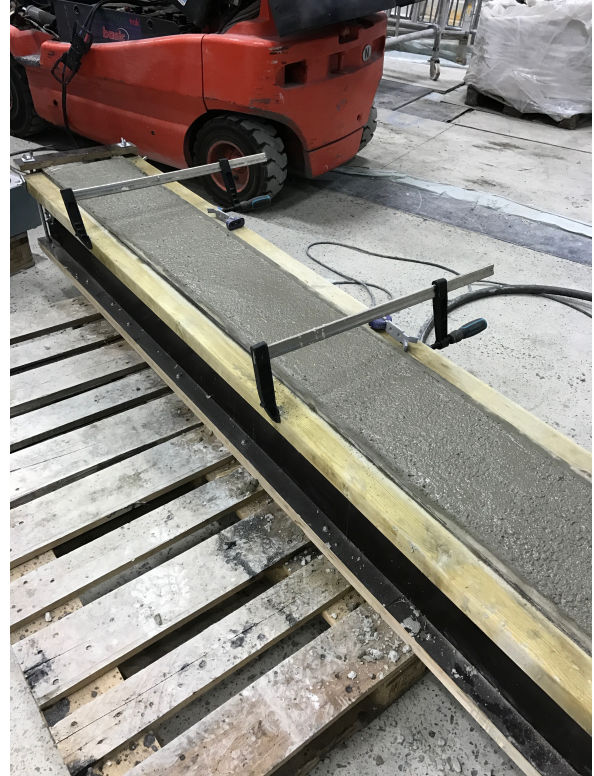
Figure 5-8: Completely casted beam.
