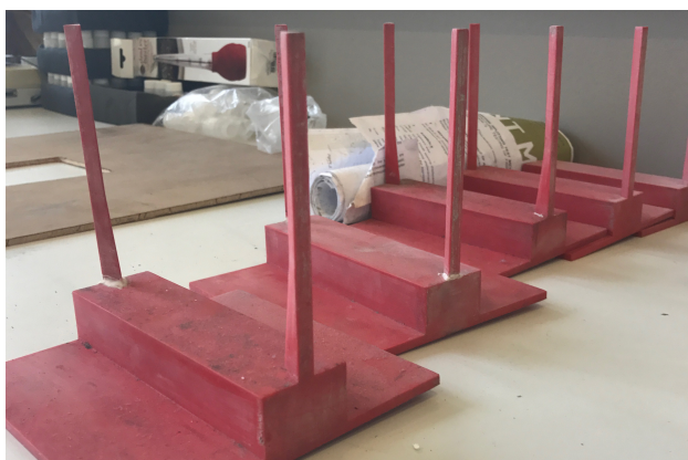
Figure 5-6: 3D-printed model made of plastic and placement in moulds
