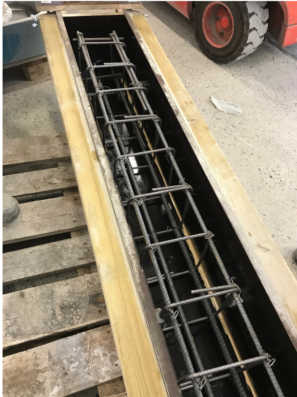
Figure 5-9: Formwork and reinforcement bars for the beam specimens.
