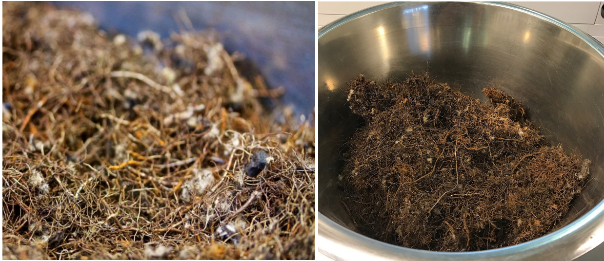
Figure 4-2: Sample of recycled steel fibres made from tyre waste
