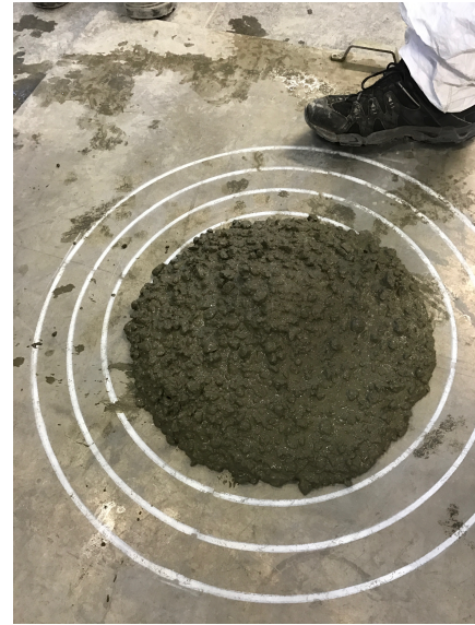
Figure 5-5: Standardized slump cone used for slump measure and slump flow test
