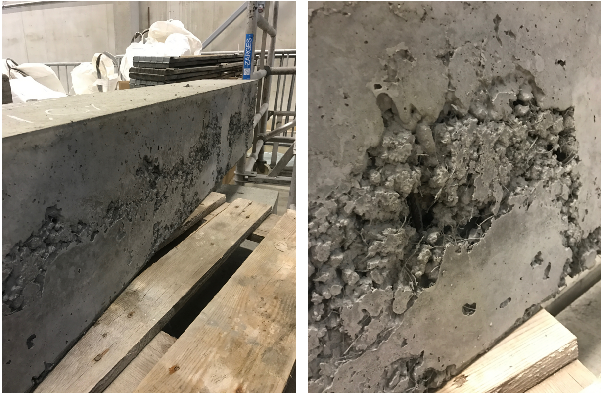
Figure 5-10: 1.0% SFRC beam with rough surface.
