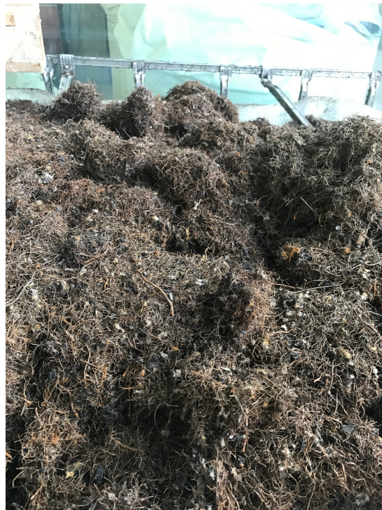
Figure 3-4: Sample of recycled steel fibres at the laboratory
